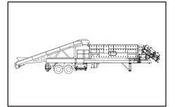
Integrated 45" feed conveyor remains on for transport and eliminates the need for a separate feed conveyor.
